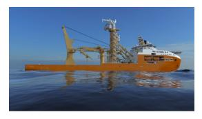
The result of an innovative design philosophy aiming to combine the installation of subsea umbilicals, risers and flowlines (SURF) with field development activities in ultra-deepwater, this new state-of-the-art offshore construction vessel, due for delivery in mid-2016, will feature a 550-tonne top tension vertical lay-system enabling the installation of large diameter flexible pipes in ultra-deepwater environments, a 900 tonne active heave
