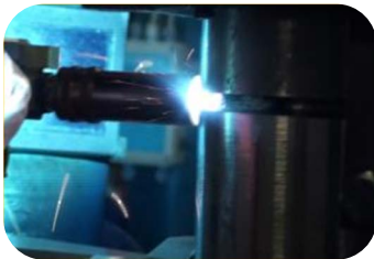
Standard steel pipe weld with inner FBJ
