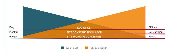
As some projects present logistic difficulties in performing work at site, the utilization of a Module Construction Approach can help to reduce the construction manhours at site thus mitigating the risk and time impact associated with site specific limitations.
