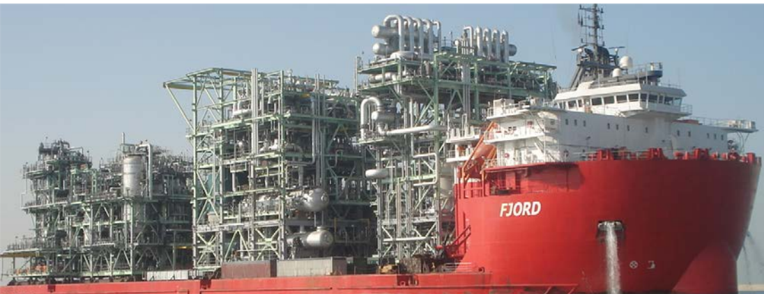
SYNGAS GENERATION COMPLEX (2X387 MMSCFD H2 CAPACITY) - GTL FACILITIES IN ESCRAVOS, NIGERIA
