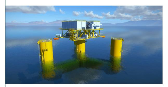
Another possible approach for the design of the floating foundation is to apply the WTG foundation design to the substation, thus providing a repeatable and scalable design for the entire wind farm. To that purpose, Saipem proprietary Star 1 and Hexafloat wind turbine floating foundation designs can be considered to support substations, focusing for the illustrations below on a rather smaller topside of approximately 350 MW capacity and 1,700 t weight.
