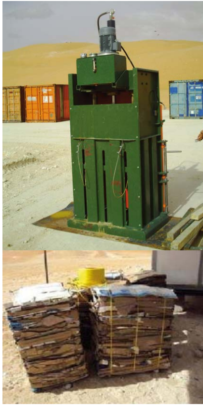
The compactor installed in the MLE project
