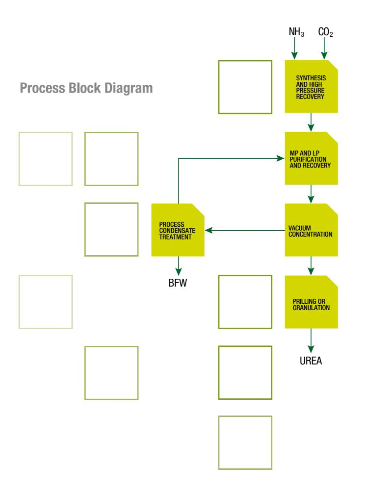
The Snamprogetti process leads to a urea solution of about 70% b.w., which is followed by a finishing step in order to obtain the solid product, either prilled or granular. Although simple, the reaction has several complex aspects:
