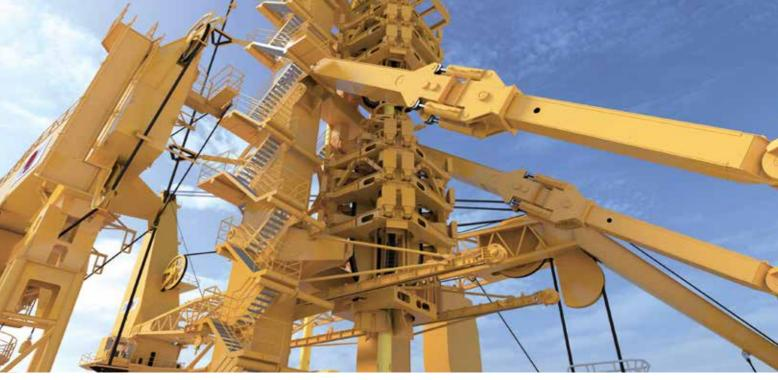
**VERTICAL LAY SYSTEM (VLS)** 550Te Vertical Lay Tower 2 X 275Te tensioners
