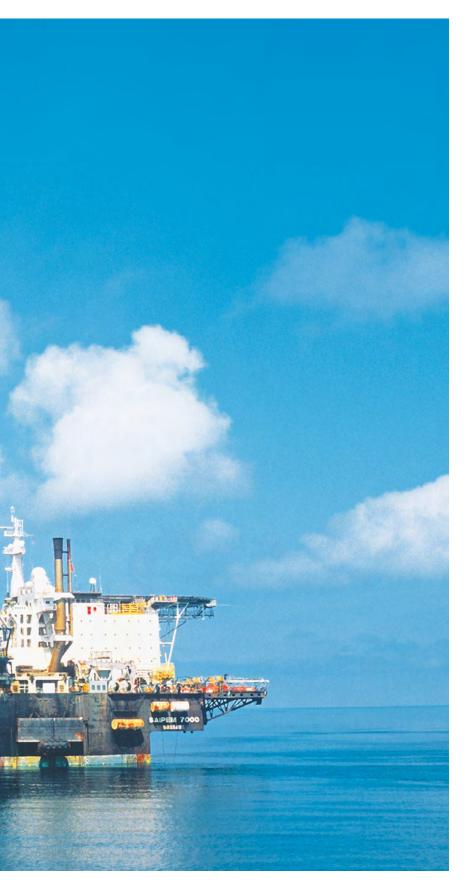
With its state-of-the-art J-lay tower, upgraded dynamic positioning capability and fast ballasting system, the Saipem 7000 semisubmersible crane vessel has the capacity to handle the entire workscope of offshore construction developments worldwide, encompassing pipelaying in water depths greater than 2,000 metres and heavy lift operations up to 14,000 tonnes.
