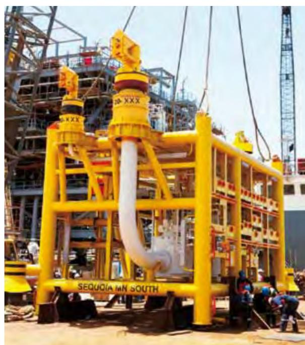
Fabrication of subsea products and equipment, such as Pipeline End Manifolds (PEM), subsea manifolds, in-line structures, well-to manifold jumpers, flowline spools and riser base jumpers, as essential complements of URF EPIC projects, allowing maximum extent of local content.
