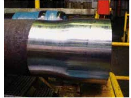
High performance thermal insulation materials and solutions including a low cost gel (here shown during filling test) for water depth down to 3,000 m, easy to fabricate in large quantities also in local yards and adaptable to any shape. This gel, under qualification, can be easily modified to serve also as a low cost buoyancy material.
