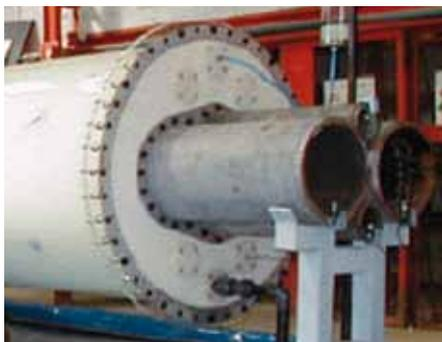
Forged Ends PIP is an innovative technology for PIP flowlines and risers, allowing an increased fatigue
