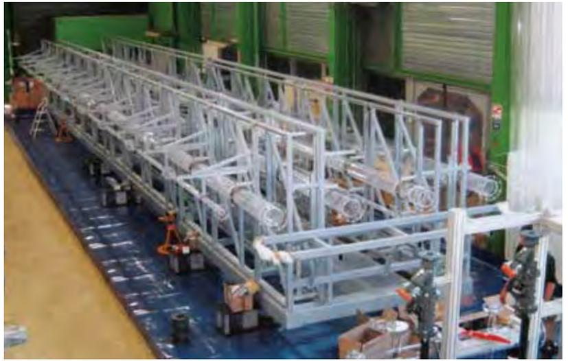
Qualification tests under way for water separation and sand management.
