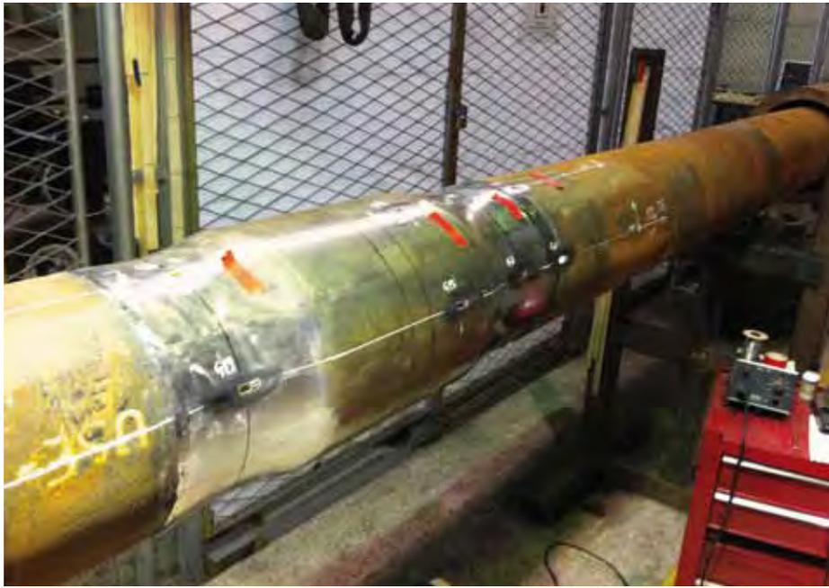
Upset & Machined End Pipes are an innovative technology developed and tested with Vallourec & Mannesman Tubes, Germany: enhanced pipe geometry to improve weld fatigue life and remove need for buckle arrestors.
