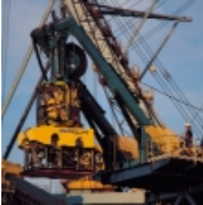
Stavanger, Norway. Innovator ROV for ultra deep water operations on board Saipem 7000.
