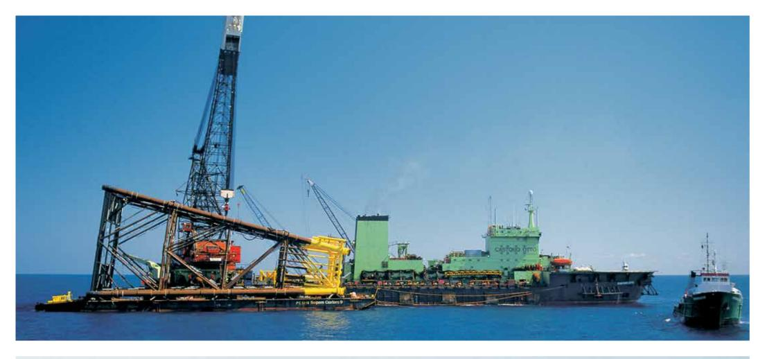
Saipem's fleet for heavy lift includes Castoro Otto and Saipem 3000 vessels, with over 2,000 t lifting capacity each.
