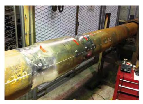
Upset & Machined End Pipes are an innovative technology developed and tested with Vallourec & Mannesman Tubes, Germany: enhanced pipe geometry to improve weld fatigue life and remove need for buckle arrestors.
