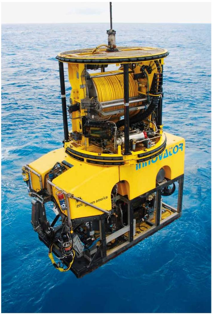
The highly versatile and powerful "Innovator" ROV's, owned and operated by Saipem, are entirely designed and built in-house
