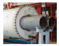
Forged Ends PIP is an innovative technology for PIP flowlines and risers, allowing an increased fatigue performance and minimization of the offshore installation time and costs.
